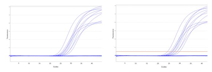
Depending on the amount of samples the linear curves should look like the ones in the picture above on the left. To set the threshold look at which cycle the first curve starts to form, in this case around cycle no. 22. Look at which cycle the first formed curve goes up in a straight line, in this case around cycle 24. See picture above on the right. The threshold is placed for demonstration purposes at the point where the curve becomes a straight line.
