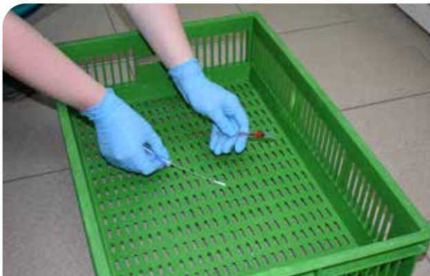
Photo 1: Sampling the surface of a transport crate with the VetAssure ATP Surface Test
